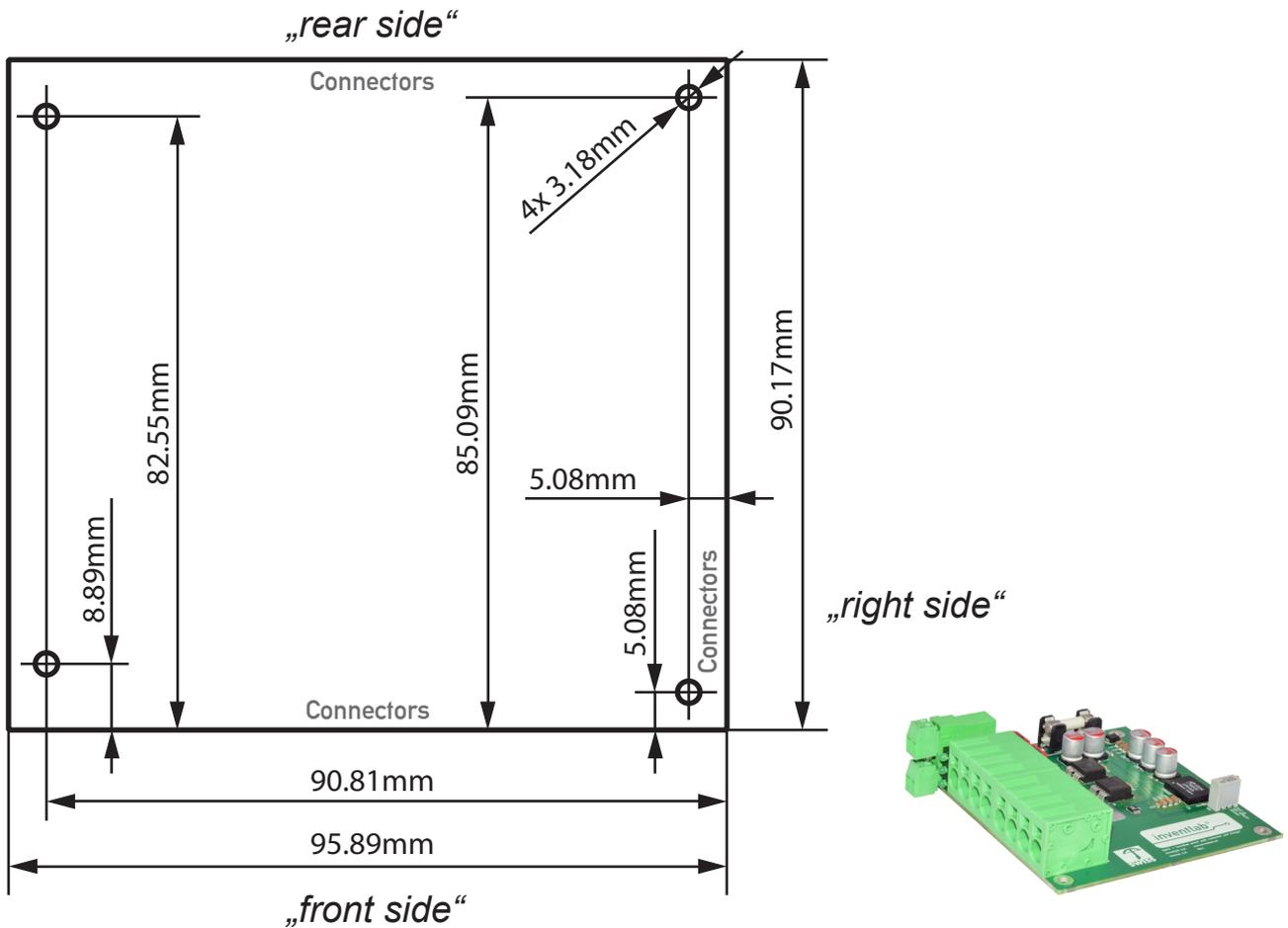
ippcc is a PC104 form factor module. All connectors and LEDs are on the „front side“. On the „rear side“ is only the voltage set potentiometer placed. On the „right side“ are no connectors.
